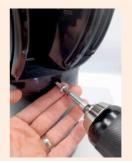
2. Anchoring the base is done through the anchor holes using appropriate anchoring techniques depending on the type of supporting structure. In the case of anchoring through thermal insulation, we will use the supplied anchor pads.
