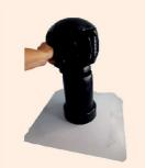
3. Subsequently, we will install the ventilation head on the vent and its trouble-free operation. The head must be mounted in a vertical position, otherwise there is a risk of uneven wear of the bearing and the turbine may not perform its function properly.
