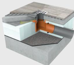
Combination of a TOPWET balcony outlet with an integrated sleeve for screed insulation and a balcony attachment with a stainless steel grid adjusted on site as required.
