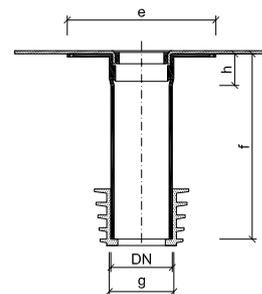
The outlet may be inserted into existing outlet, pipe or gutter up to a neck, but it has lower drain capacity
