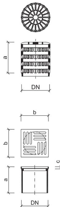
\* How can attachments be universal for various diameters of roof and terrace outlets DN 50, 70, 100 and 125?
