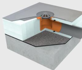
Combination of a TOPWET balcony outlet with an integrated sleeve and a flat walkable protective basket supplied as standard with balcony outlets.
