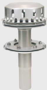
LORO waste piping from hot-dip galvanized steel with an internal layer from two-component epoxide of reddish brown colour with a deep flange for connecting pipes, supplied without an O-ring. The piping DN 50–150 is supplied in the length from 250 to 3000 mm.
