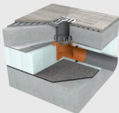
Combination of a TOPWET balcony outlet with an integrated sleeve and balcony attachment with a stainless steel grid and a drainage ring used for water drainage from the main hydro-insulation layer.
